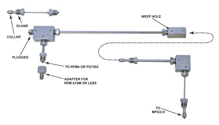
Figure 1: Nipples installed in 3-way tee, elbow and union
